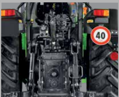
Powerful hydraulic system with a capacity of up to 60 l / min
