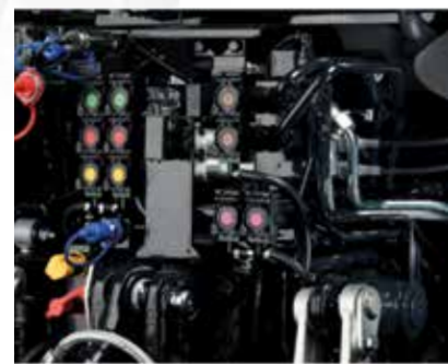
Hydraulics. 120 L/min capacity closed- centre hydraulic system
