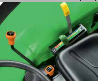
Wet clutch Power Shuttle with 3-stage ECO-Speed Powershift transmission (45x45)
