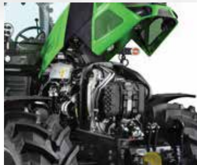
Tier 3 FARMotion Engine 4-cylinder turbo intercooled
