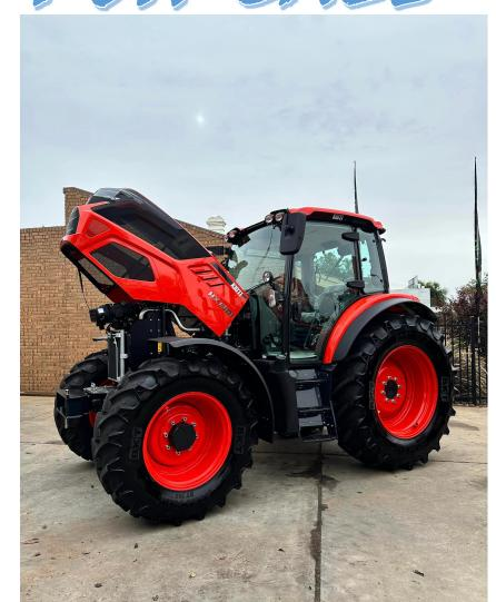
130 hp 8 Speed Powershift Auto Powershift 32 x 32 Transmission Limited Slip Differential Closed Centre Hydraulics Multi-Functional Armrest With loader and Bucket
