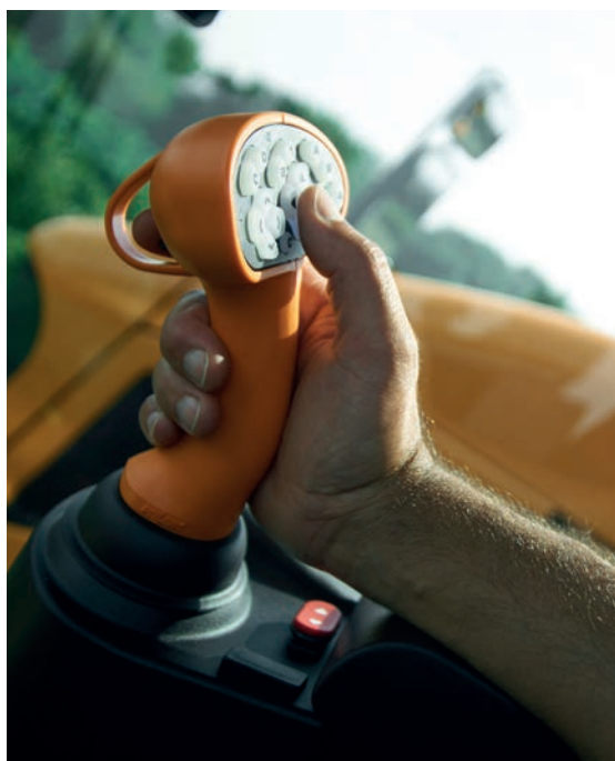
Tool control from the EASY DRIVE Joystick
