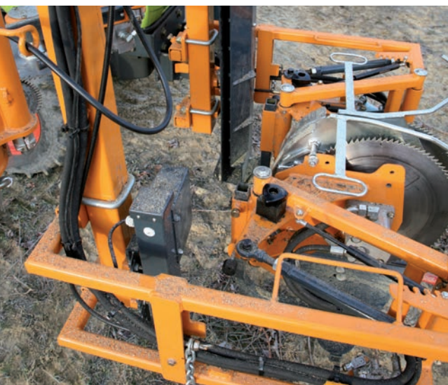
Automatic cordon tracking by vision system.
