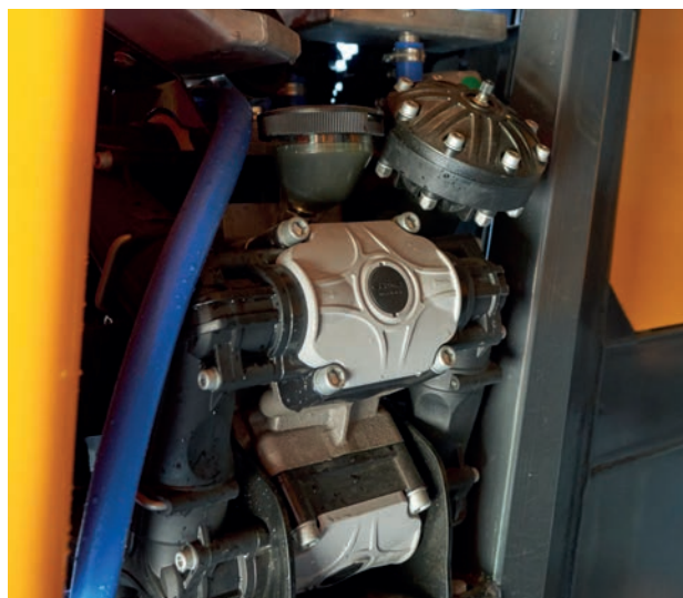
Variable flow pump, up to 260 litres/min.
