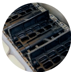
Flexible sorting conveyor
