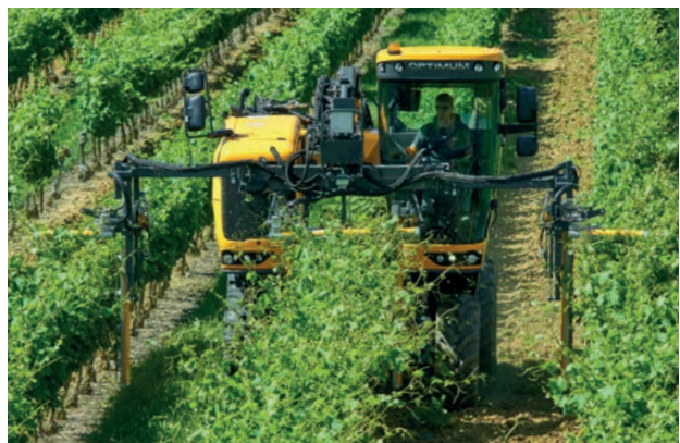
Trimmer on the multifunction arm
