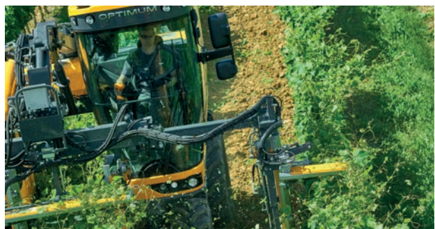
Trimmer on the multifunction arm
