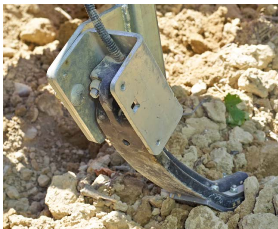
Ground probe of the tool holder arm
