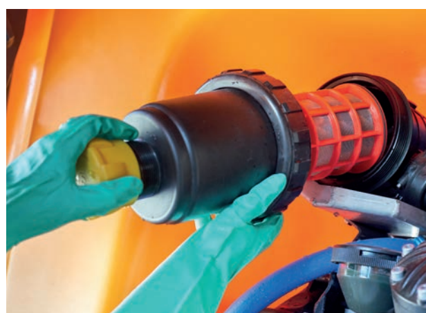
Easy disassembly of filters
